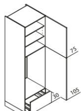
**GKA Appliance unit for refrigerator / recess 102.5 cm**
