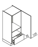
**GKA Appliance unit for refrigerator / recess 88 cm**
