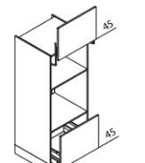
**GBLA Appliance housing with lift-up door for oven and microwave**
