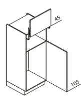
**GKL Appliance housing with lift-up door for refrigerator / microwave / recess 88 cm**
