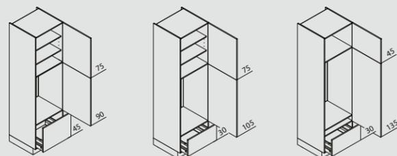
By way of example, an appliance housing for a refrigerator in 21 cm height with recess heights of 88, 102.5 and 122.5 cm (from left).
