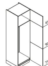
**GKG Appliance unit for refrigerator / freezer combination / recess 158 cm**
