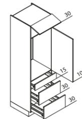
**GKAK Appliance unit for refrigerator / recess 102.5 cm**
