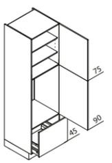
**GKA Appliance unit for refrigerator / recess 88 cm**
