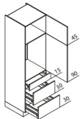
**GKAK Appliance unit for refrigerator / recess 88 cm**
