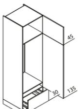
**GKA Appliance unit for refrigerator / recess 122.5 cm**
