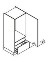
**GKA Appliance unit for refrigerator / recess 102.5 cm**
