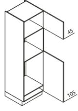
**GKB** Appliance housing for refrigerator and oven / recess 88mm
